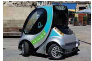
The Hiriko, an electric car specially developed for cities by the Massachusetts Institute of Technology, folds up so that three cars can fit into one parking space.
